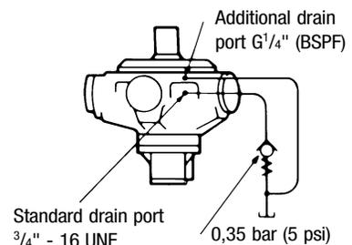
An additional G<sup>1</sup>/<sub>4</sub>" (BSPF) drain port in the front cover is provided when the “V” (shaft vertically upwards) designator is given after the shaft type letter in position **3** of the model code. This additional drain should be connected into the main motor casing drain line downstream of a 0,35 bar (5 psi) check valve to ensure lubrication of the upper bearing, see above diagram.
