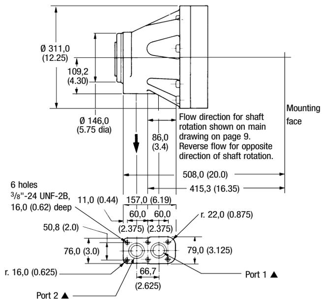
▲  $\varnothing 38,1$  (1.5 dia), with recess for 38,1 (1.5) i/d x  $\varnothing 3,53$  (0.139 dia) section O-ring
