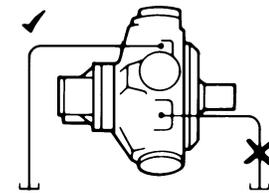
The crankcase drain must be taken from a position above the horizontal centre line of the motor.
