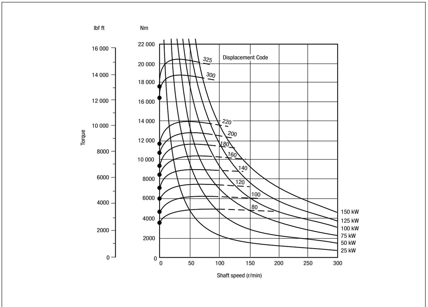
The torque curves indicate, for each displacement, the maximum output torque of the motor with an inlet pressure of 250 bar (3626 psi) and zero output pressure. High return line pressure will reduce the torque for any given pressure differential.
