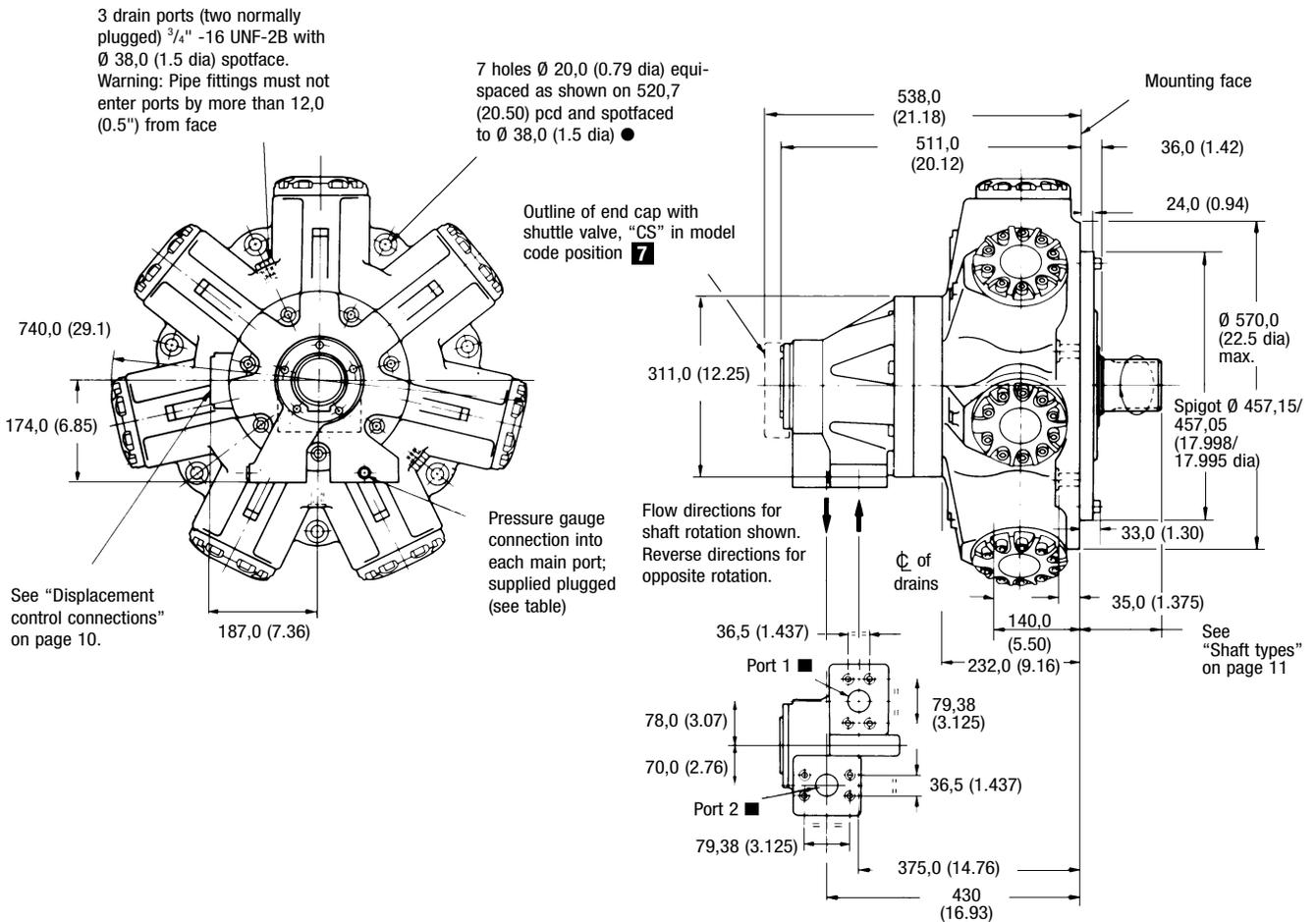
● Suitable for M20 or 3/4" bolts. Maximum reaming diameter 21,0 (0.83) (for fitted bolt); see "Installation Data".
