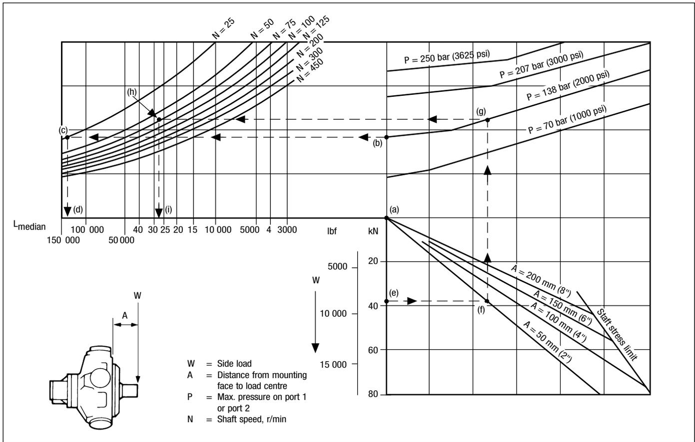
The nomograph allows the median bearing life to be determined for conditions of:
