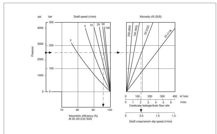
This nomograph enables the average volumetric efficiency, crankcase (drain) leakage and "winch slip"/shaft creep speed to be estimated.
