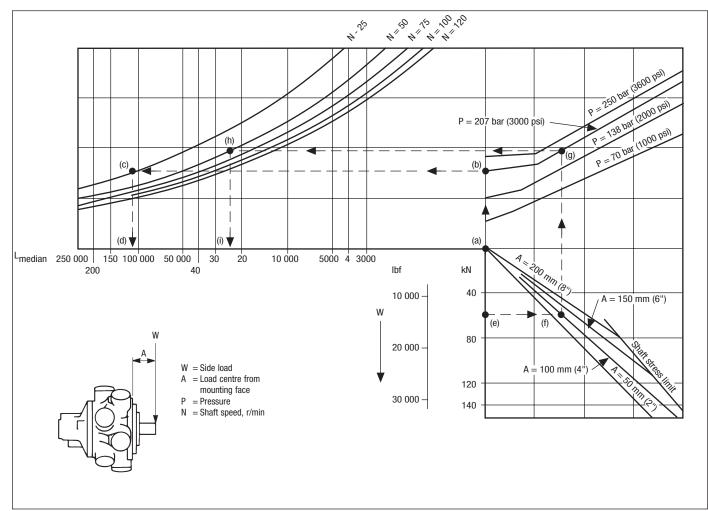
The nomograph allows the median▲ bearing life to be determined for conditions of:
