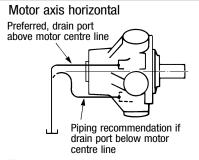
The motor should be installed with the drain port above the shaft centre line to ensure adequate lubrication of the bearings. When this is not possible and the drain port is positioned below the shaft centre line, the drain line should be run to at least the level of the shaft centre line; see above diagram.
