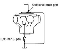
An additional drain port is provided when the "V" (shaft vertically upwards) designator is given after the shaft type letter in position of the model code. This additional drain should be connected into the main motor casing drain line downstream of a 0,35 bar (5 psi) check valve to ensure lubrication of the upper bearing.
